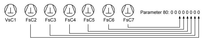
Example: In a rack system with one Variable-speed Compressor (VsC1) and two Fixed-speed Compressors (FsC2 & FsC3) parameter 80 has to be set to: 00000011
